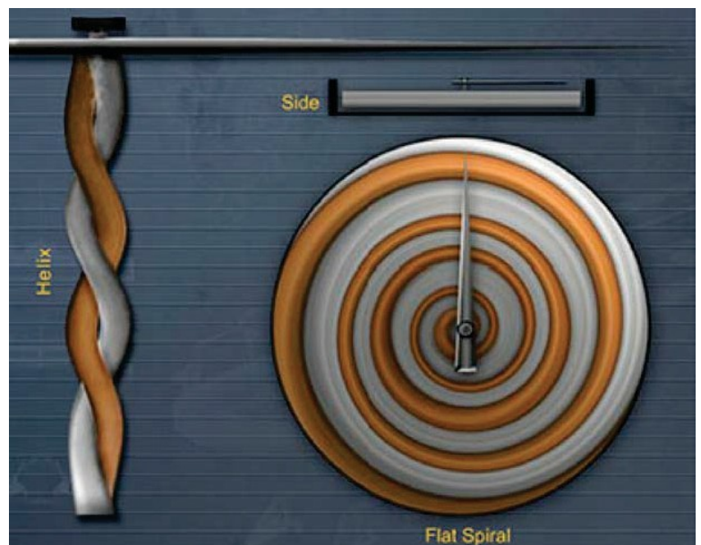
Figure 11-12 — Bimetallic thermometer (flat, spiral strip).
