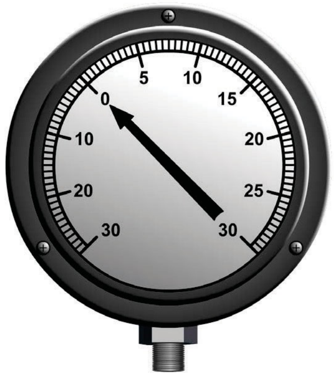
Figure 11-5 — Compound Bourdon-tube gauge.
